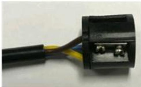
4. Plug another side wires, make sure the wires colors are correspondingly, then screw tightly
