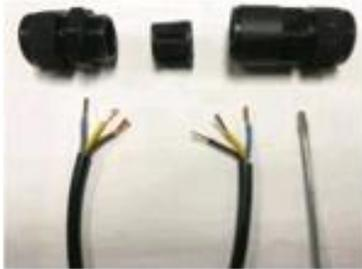
2. Back out the screws on conductor a little, make the hole enough to plug wire in
